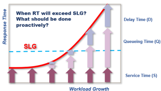
Figure 9. Modeling results predict how different changes will affect the major components of the Response Time, Throughput and resource utilization by each workload
